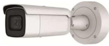
Cámara IP 8 Megapixel 1/2.5" Progressive Scan CMOS. Compresión H.265+/H.265/H.264+/H.264. Lente motorizada AF 2.8~12 mm Autofocus IR LEDs Alcance 50 m | Audio y Alarmas. Interfaz WEB, CMS, Smartphone y NVR.
